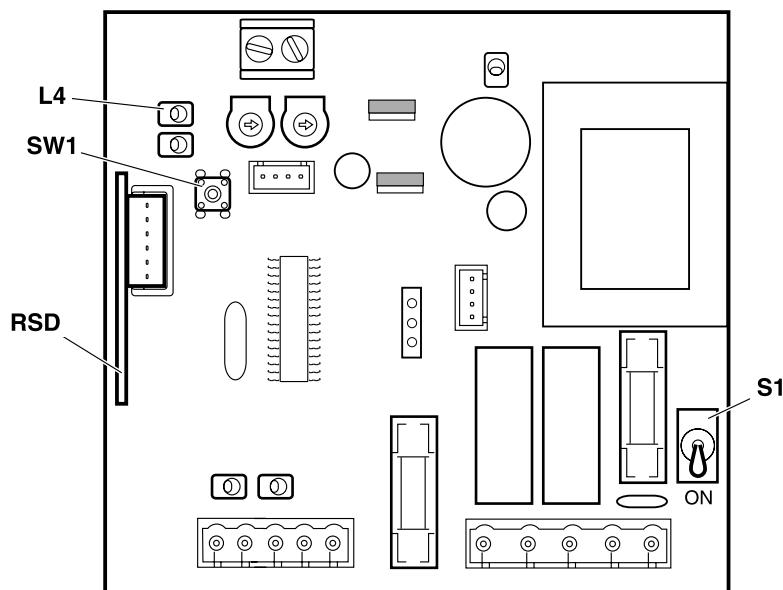
When using Fixed Code transmitters (433.92MHz or 868.35MHz) and the RSD-433 (433.92MHz) or RSD-868 (868.35MHz) plug-in receiver, the radio code can be saved in the control board itself, as explained below. In other cases, follow the instructions of the plug-in receiver used.
